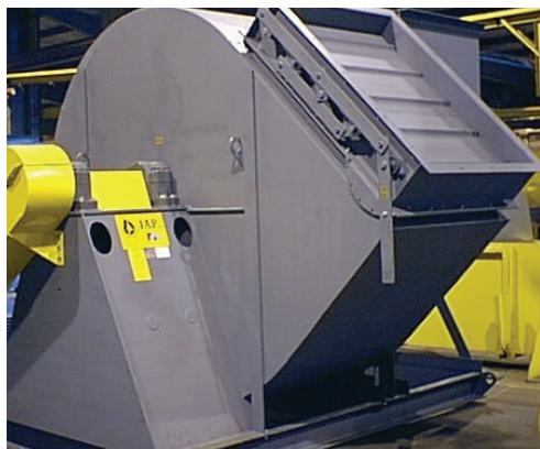
Double wall clad housing, above & below
