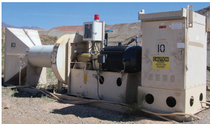
Mine shaft pressurization (above); single skid mounted inlet filter box, silencer, blower assembly, disconnect and power supply drive. Multiple units, shown below, during factory assembly.
